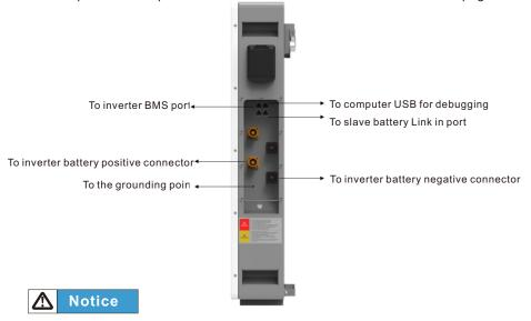
Please debug battery by engineer software before recovering operation plate.
